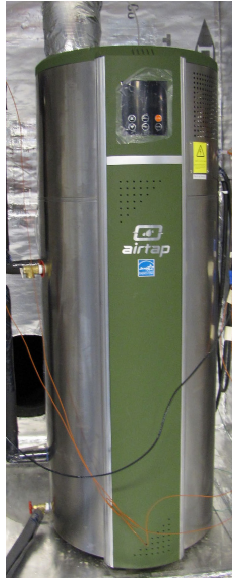
Heat Pump Water Heater technology has the potential to save twice as much energy when compared to an all-electric water heater because it utilizes the heat in the surrounding air instead of relying solely on electric resistance to heat the water. Photo by Kate Hudon for NREL.
