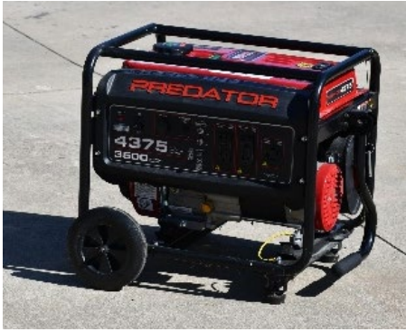
▲ The only safe way to connect a portable generator to your home is by using a transfer switch. Photo courtesy of SafeElectricity.org
