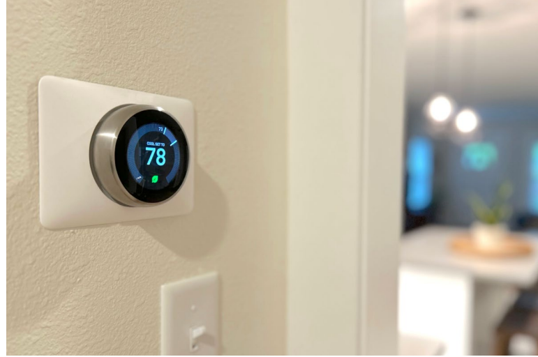
Smart thermostats offer a variety of bells and whistles, but the average model will allow you to set custom temperature schedules, adjust the settings from anywhere, and over time, learn your cooling and heating preferences. Photo Source: Abby Berry, NRECA
