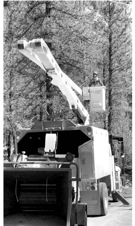
▲ Once a tree is cut and limbed in sections from a bucket truck, debris is fed into a chipper, which feeds into a dump truck. The chips are then hauled away.
